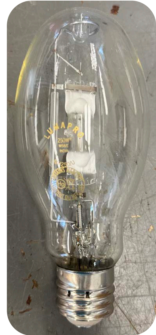
A 250W, 22,000 Lumen, HID metal halide lamp – 4,000K
